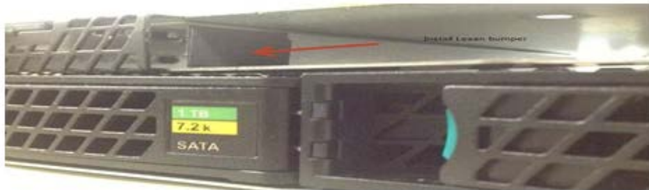
Figure 2. Example of the Mylar on the side of the DVDROM bay
