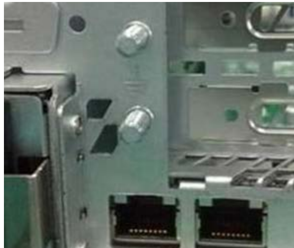
Figure 1: The ground studs
