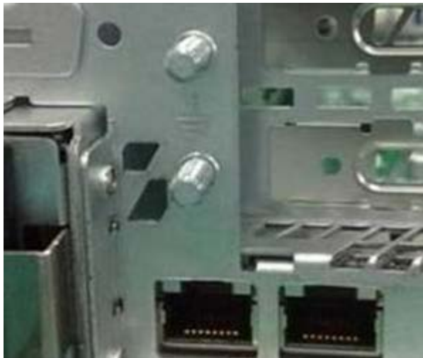
Figure 1: The ground studs
