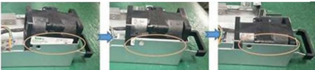
Figure 3. Label is now covered and protected by power supply chassis
