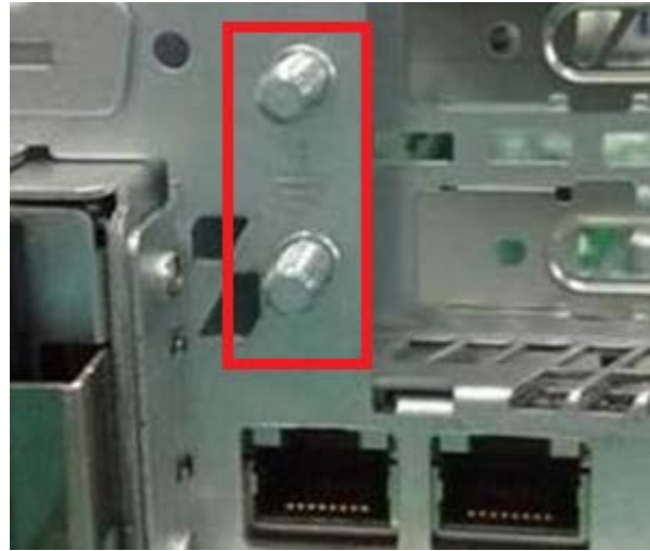
Figure 1: The ground studs
