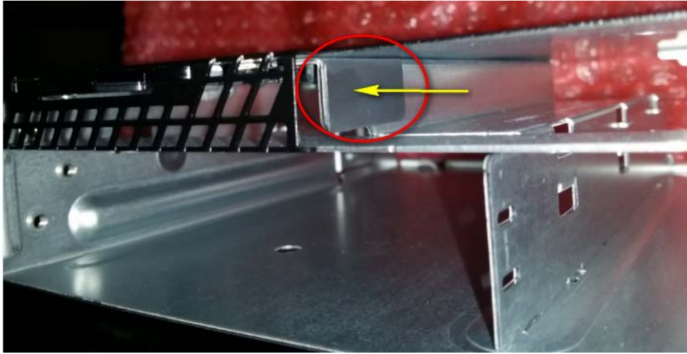
Figure 6. Example of the mylar bumper on the side of the optical drive bay.
