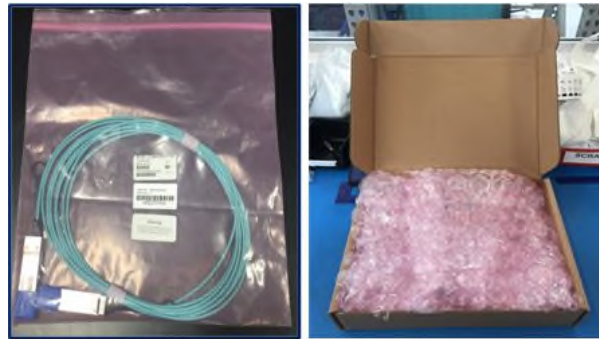
Figure 3. AOC Cable in a Single-Box with Foam Insert (Updated Method)
