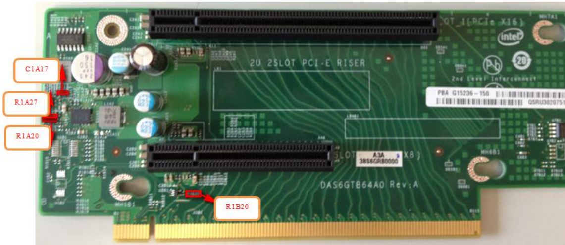
Figure 2 Component Locations for the 2U Riser Spare A2UL16RISER
