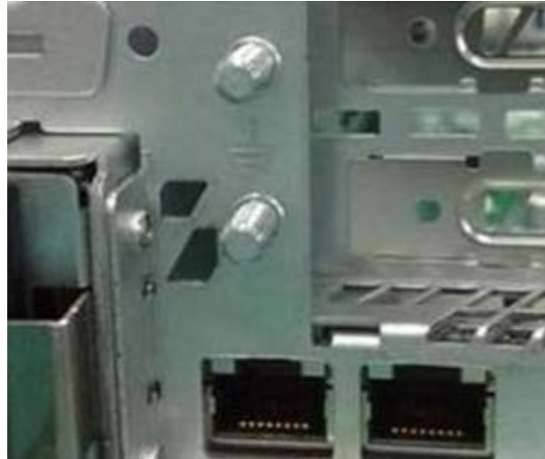
Figure 1: The ground studs
